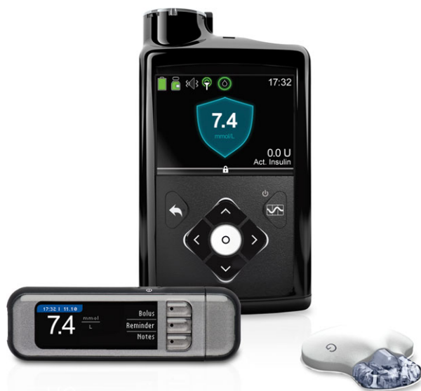
FIGURE 3 Hybrid closed-loop system comprising fourth generation Enlite 3 glucose sensor, MiniMed® 670G insulin pump, with an embedded proportional-integral-derivative algorithm with insulin feedback (Medtronic, Northridge, CA, USA). Reproduced with permission from Medtronic.
